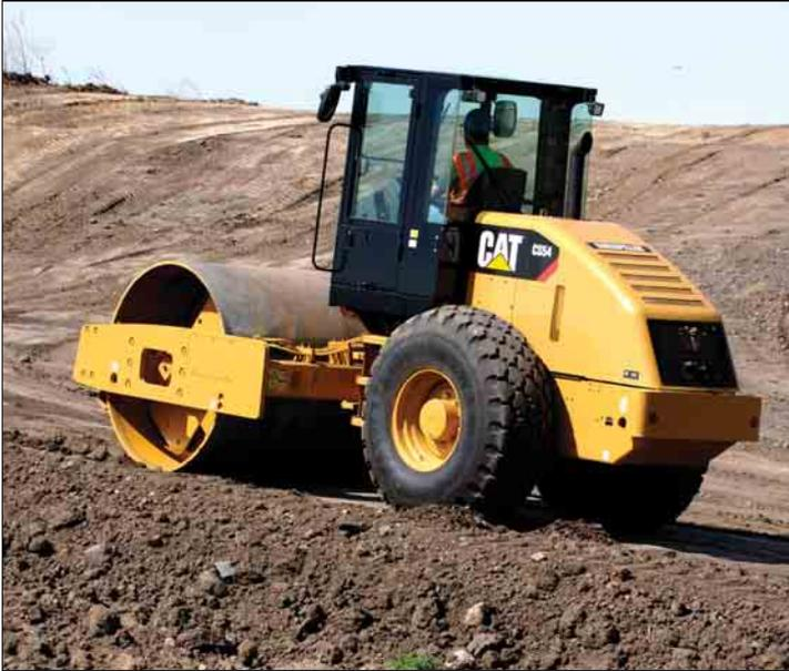
**Propel pump system.** The dual propel pump system has dedicated pumps to independently drive the heavy-duty, high-torque rear wheel and drum motors. Should the drum or wheels begin to spin, the non-spinning motor still receives hydraulic flow, allowing continuous tractive effort especially useful in loose underfoot conditions.
